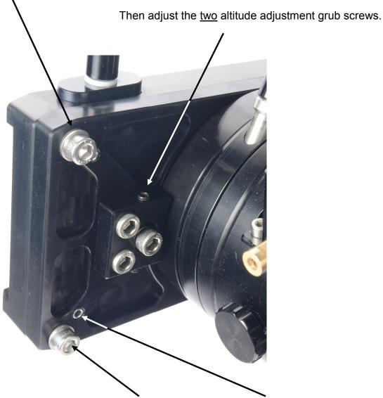
Slight adjustment in azimuth is also possible by adjusting the 4 x grub screws on the corner of the adjustment plate. This has to be done in co-ordination of the M6 bolts.
