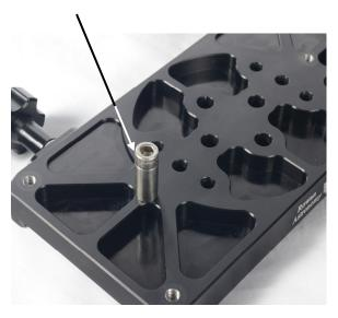
4) Fit the saddle to the adjustment plate with the M6 x 20 bolts and washers, leave slack.
