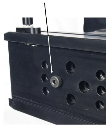
6) To make altitude alignment adjustment, 'slightly slacken' the 4x M6 bolts.
