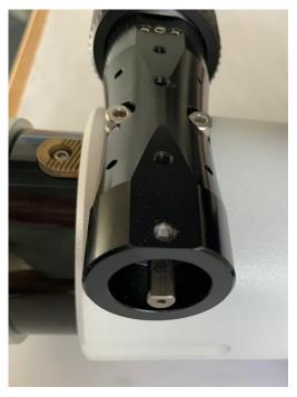
Then, turn the focus wheel until its hex screw appears in the thread bore of the removed setting screw. Loosen it. In some cases, there is a second setting screw in a 90° position. Loosen it, too. Now you can pull off the focus wheel.
