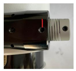
Take the correct coupling for the shaft diameter out of the EAF box and tighten both screws through the bore (tighten first one, turn the shaft by 90° and tighten the other one).
