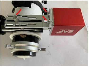
Now, fix the holding bracket loosely to the focus motor and align it to the focus mechanism with the motor shaft inside the coupling. Use the original locking screw to fix the bracket and tighten the bracket screws (right red marks) if everything is in place. Tighten also the setting screws at the motor side of the coupling.
