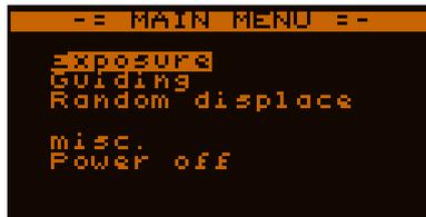
Certain items behave differently. There are *number*, *time* and *text* types etc. Text type items can lead to a submenu or are to do some function (like a button), while other (*number* or *time*) types store a value that could be edited/changed and are called *parameters* or *variables*. These are to setup, parametrize the device, to control its behaviour.
