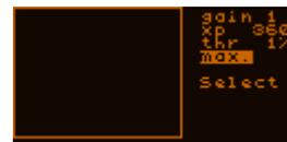
The value of most of the parameters or variables are stored into EEPROM memory of the HC at power-off. At the next power-on they are initialized from here.
