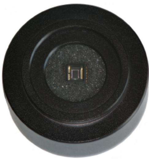
To attach the Camare to the guider telescope there is a 4-5mm thick T2 inside screw. Any T2? 1.25" adapter can be used for 1.25" (31.7mm) focusers. There is a 1.25" filter thread inside the T2 panel to attach some filter or "dust preventor".
