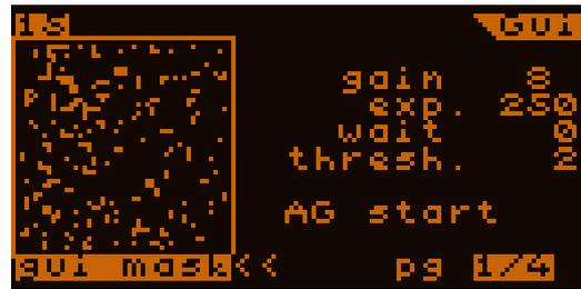
On the Guiding screen there is always the guiding star (or other) monitored in the window on the left. This is a 48x48 pixel window in a frame.
