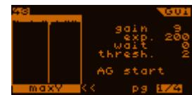
Note: the diagram is NOT a histogram but a “vertically projected map” of the raw image. This mode is used to trim the focus precisely. If the diagram shows a wide ‘hump’ the star may be out of focus. The focus is the best if the thickness of the hump is the smallest and the rise of the sides are the highest.
