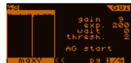
Note: the diagram is NOT a histogram but a “vertically projected map” of the raw image. This mode is used to trim the focus precisely. If the diagram shows a wide ‘hump’ the star may be out of focus. The focus is the best if the thickness of the hump is the smallest and the rise of the sides are the highest.
