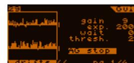
should be held. The latest 48 drift values are shown for the latest 48 frames, for each axis. One time step (one frame) is one pixel horizontally while vertically the drift values are scaled to the tolerance limit set. The tolerance is shown right next to the frame with two short lines, the size of it is  $\pm 2$  pixels to the zero.
