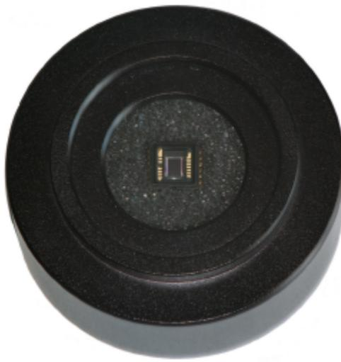
To attach the Camera to the guider telescope there is a 4-5mm thick T2 inside screw. Any T2? 1.25" adapter can be used for 1.25" (31.7mm) focusers. There is a 1.25" filter thread inside the T2 panel to attach some filter or "dust preventor".
