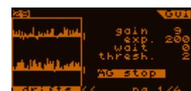
should be held. The latest 48 drift values are shown for the latest 48 frames, for each axis. One time step (one frame) is one pixel horizontally while vertically the drift values are scaled to the tolerance limit set. The tolerance is shown right next to the frame with two short lines, the size of it is  $\pm 2$  pixels to the zero. As the tolerance value is changed so changes the appropriate axis' drift diagram's scaling.
