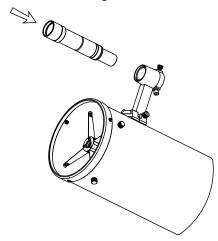
remove the dust cover and Loosen the thumbscrews on the end of the focuser adapter.
