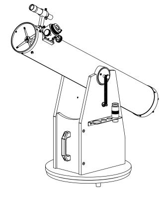
Loop the cord provided through the hook on one end of the spring.
